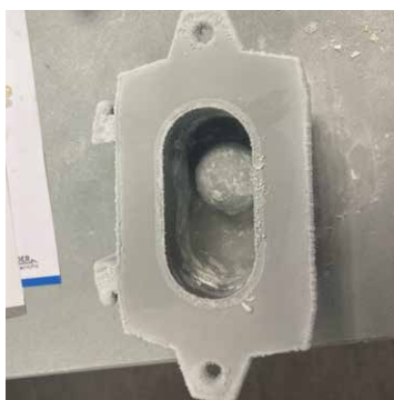
Fig. 3: 125 ml jar with balls and frozen pellet (above); 50 ml jar, after sample retrieval (below)
