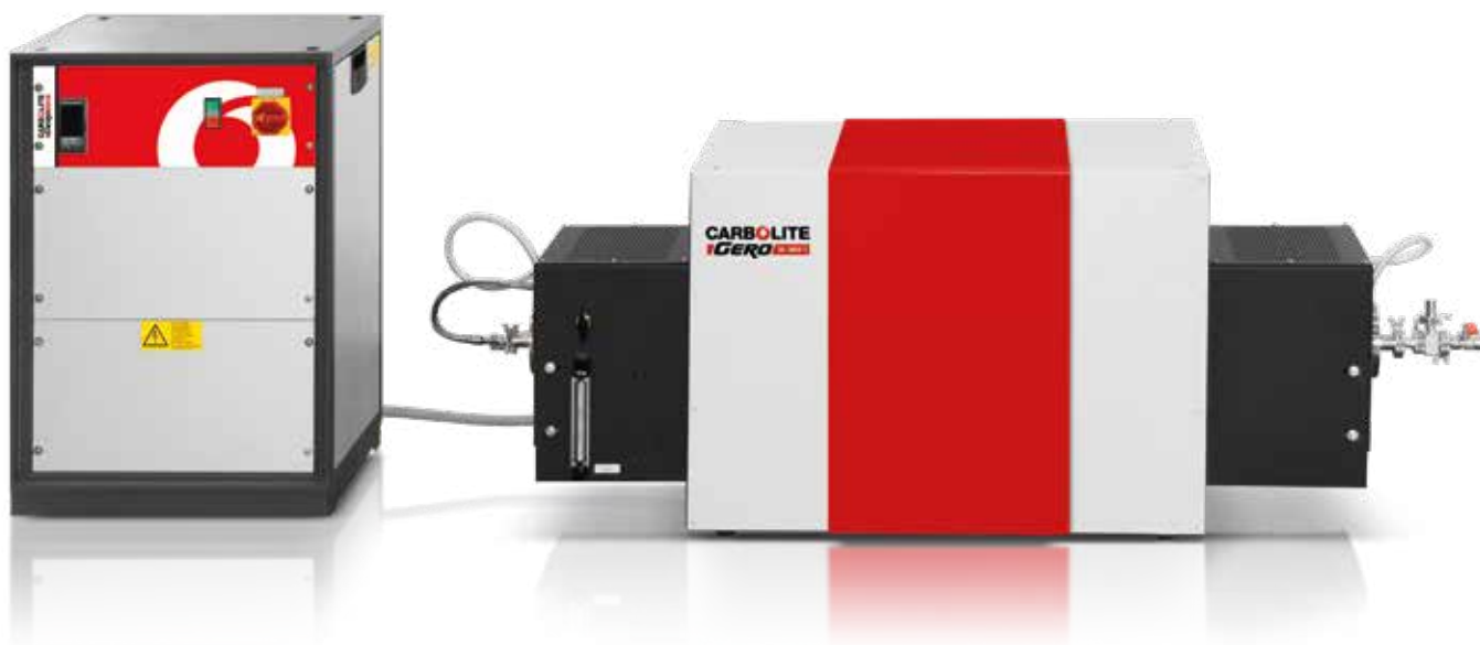
Horizontal High Temperature Tube Furnace HTRH 18/70/600 with optional EPC3008P10 programmer and optional high vacuum capable inert gas package (high vacuum capable up to 1450 °C and up to 1800 °C under normal pressure). Rotary vane pumps and turbo pumps optional available (see page 106).
