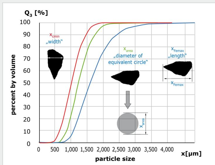
Fig. 5: Different size definitions in dynamic image analysis provide different results for non-spherical particles.
