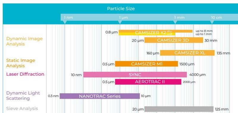
Fig. 1: Measuring ranges of different methods
