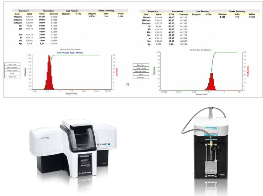
Fig. 14: Size distribution of a barium sulfate suspension measured with laser diffraction (Microtrac SYNC) and DLS (Nanotracs Flex). The matching of the measured values is excellent, the median is 138 nm.
