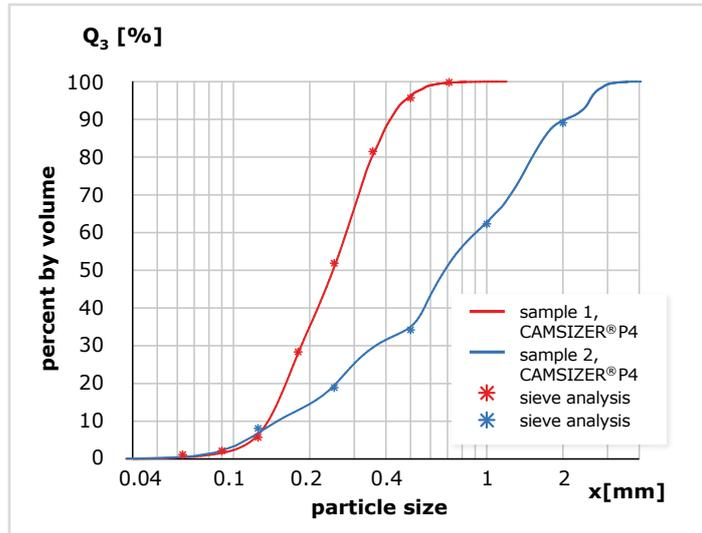
Fig. 7: Good comparability of image analysis and sieving results for wide and narrow distributions thanks to material-specific fitting function.
