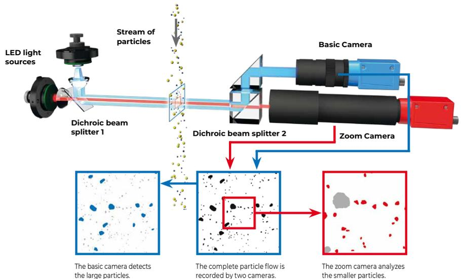
The particles can be in free fall, in suspension in a liquid, or, if they tend to form agglomerates, dispersed (separated) by compressed air. Modern DIA systems evaluate several hundred images per second and capture many millions of individual particles within one measurement. Fast cameras, bright light sources, short exposure times and powerful software are the prerequisites for this.
