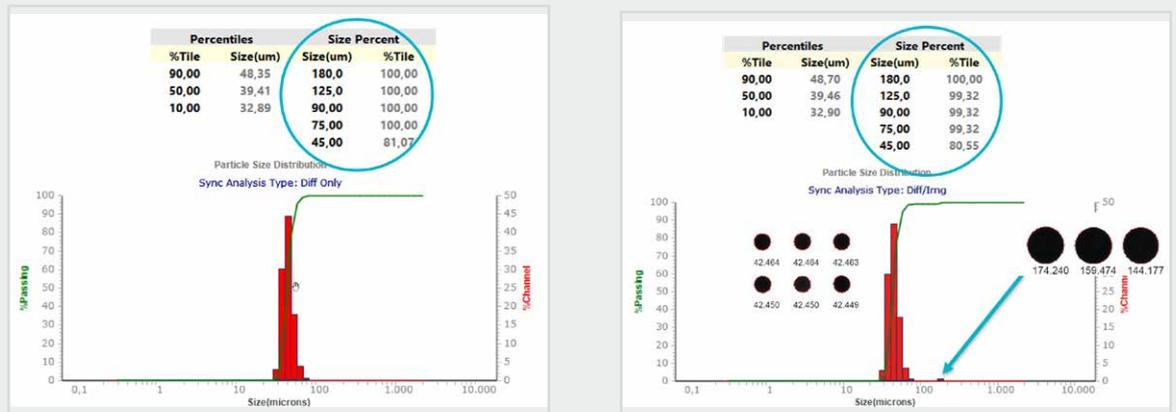
Fig. 12: Oversize detection. Oversize grains were added to a sample of metal powder in a controlled manner. Left: Laser diffraction alone cannot detect oversize contained in the sample. Combining this with image analysis in Microtrac SYNC detects and displays 0.5% oversize. Bottom: a pure image analysis instrument like the CAMSIZER X2 can still correctly measure oversize particles even in low concentrations like 0.005 %.
