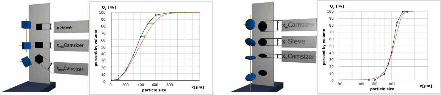
Fig. 6: Typical differences between dynamic image analysis (red) and sieve analysis (black) for approximately angular, cube-shaped material and more platy material.
