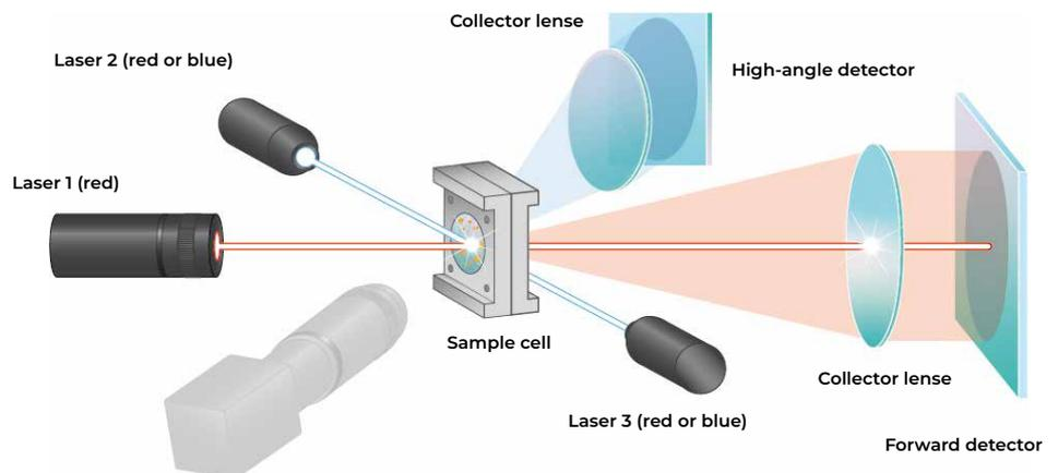
Fig. 9: Setup of the SYNC laser particle analyzer. The sample in the measuring cell is detected by three lasers from different angles. The resulting scattered light is recorded by two detector arrays over a total angular range of 0.02° to 163°.
