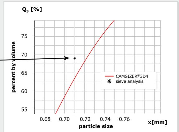
Fig. 8: Minor differences between image analysis (red) and sieving (black) for spherical particles can be explained by sieving tolerances.
