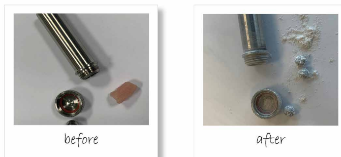
Figure 4: Homogenization of frozen tissue in the MM 500 control at -60\text{ }^{\circ}\text{C} .
