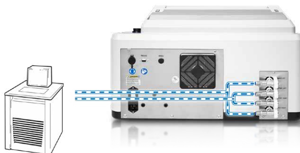
Figure 2: Setup 1 - Cooling with a recirculating chiller.
