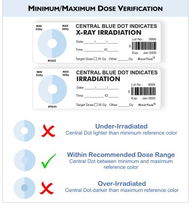
RadTag<sup>®</sup> indicators are specially calibrated to verify that the dose of irradiation delivered falls within recommended ranges and that irradiated blood is safe to transfuse.
